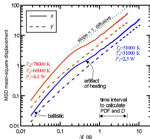
FIG. 2 (color online). MSD, averaged over threads and overlapping time segments [34], computed separately for  $x$  and  $y$ . Data here are for two laser powers. The MSD in the  $x$  direction is larger than that in the  $y$  direction, due to  $T_x > T_y$ . Distance is normalized by the Wigner-Seitz radius  $a$ .
