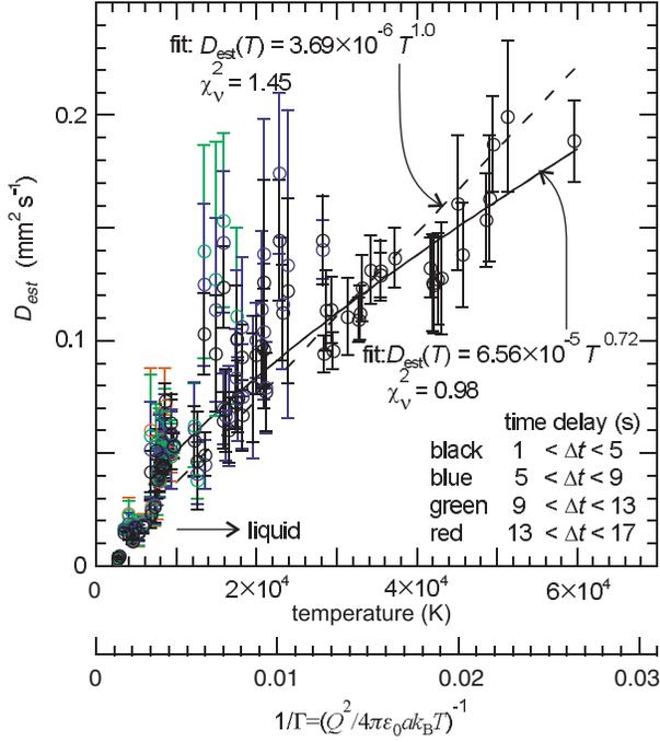
FIG. 4 (color online). Temperature dependence of  $D_{\text{est}}$  calculated from  $\langle (y(\Delta t) - y(0))^2 \rangle / 2\Delta t$ . The smooth curve is a fit, weighted by error bars, of data for a liquid. Scatter is due to finite time interval and number of threads.
